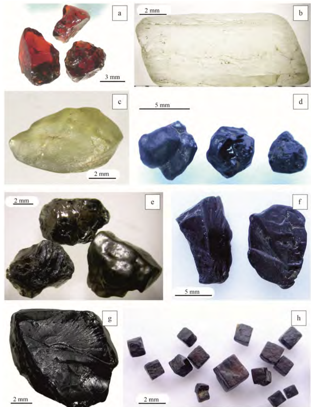
Figure 9. Minerals of the Naryn-Gol placer. (a)—garnet, (b)—feldspar, (c)—olivine, (d)—spinel, (e)—orthopyroxene, (f)—clinopyroxene, (g)—ilmenite, and (h)—pseudomorphs after pyrite.
