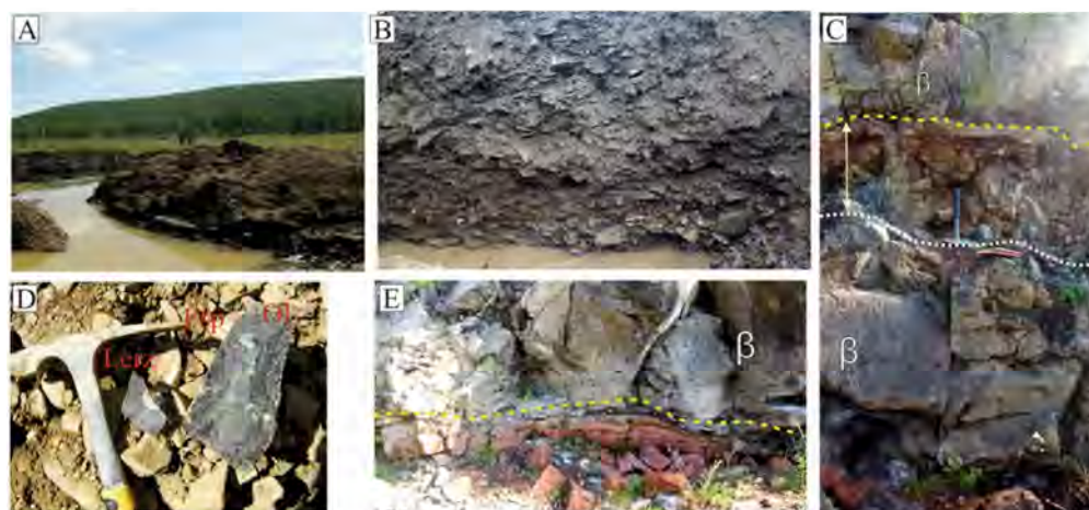
Figure 2. Trenches and test pits in the Naryn-Gol Creek placer. (A)—exposed permafrost layer; (B)—gem-bearing bed; (C)—residual weathered layer and pyroclastic rocks covered by basaltic flows; (D)—poorly rounded basaltic corestone containing lherzolite xenoliths and megacrysts of olivine and sanidine; and (E)—basalt flow overlying the residual weathered layer exposed at the base of the Cenozoic volcano. \beta —basalts; Lerz: lherzolite; Fsp: feldspar; Ol: olivine.
